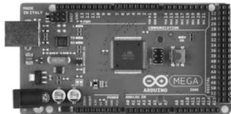
Gambar 9. Arduino Mega 2560
